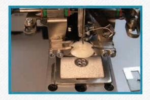
Backing button plate can be instantly changed by the operator
