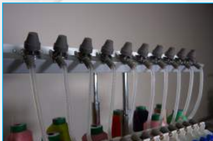
Easy and smooth threading tube
