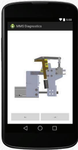
Various other screen can be easily accessed. This screen shows the diagnostics page for the thread bonding device. By touching the various components on the screen the actual components will move inside the machine. Other screens give the possibility to pre set the 3 programs, alter the bonding time and update the software. Many more features will be built in as time goes on and these will be updateable via the MMS APP.
