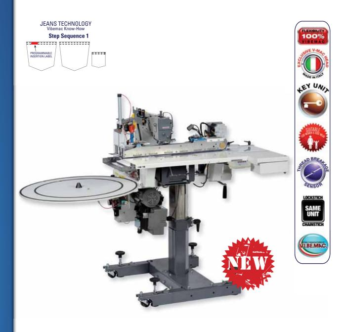
The V701 is a 2011 brand new unit and the solution to many productivity & quality problems that might occur when performing the first step in the jeans production, hemming the back pockets.
